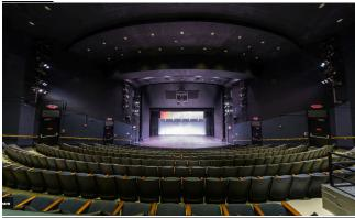
Extended apron stage with 21'-0" deep apron located at bottom of steeply stepped house. Stage floor is black hardboard over plywood over concrete, in good condition. A 360-degree video of the stage is available at: youvisit.com/tour/panoramas/60013/80305?id=211052. Select Shea Auditorium from the scroll bar on the right.
