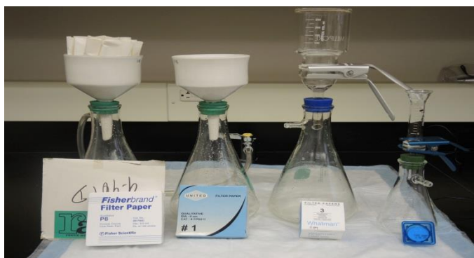
Figure 2. The filtration set-up for generating the weathering solutions.
